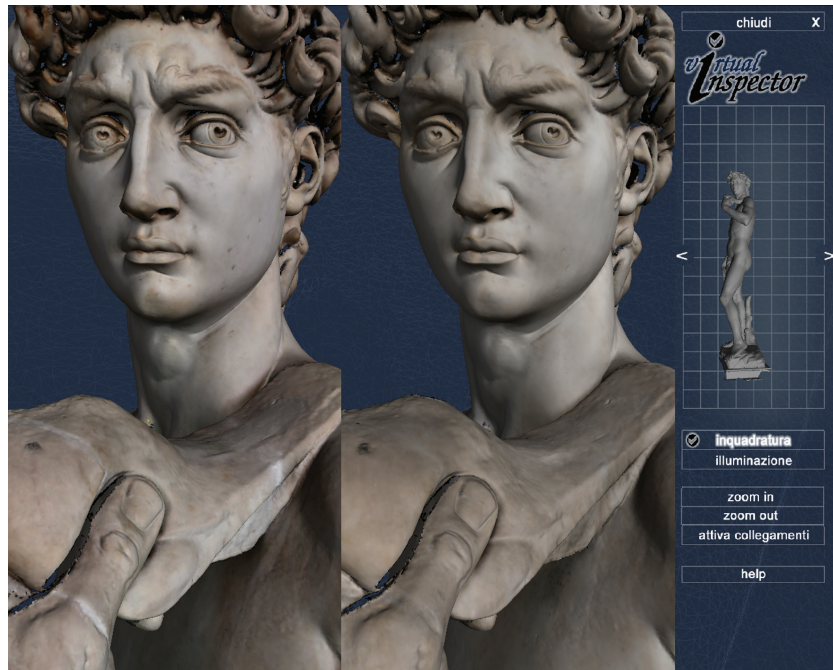
Fig. 6. The David model is shown with color mapping. On the left is the prerestoration status (61 images mapped), while the postrestoration status is shown on the right (another set of 68 images). The two-colored David models are rendered in real time with the Virtual Inspector system.
