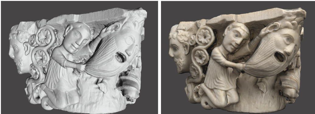
Fig. 2. A 3D scanned model (laser triangulation) of a medieval capital (S. Matteo Museum, Pisa, Italy). On the left is the digital model rendered as a standard grey surface, while the image on the right is rendered after mapping color detail to the 3D mesh.
