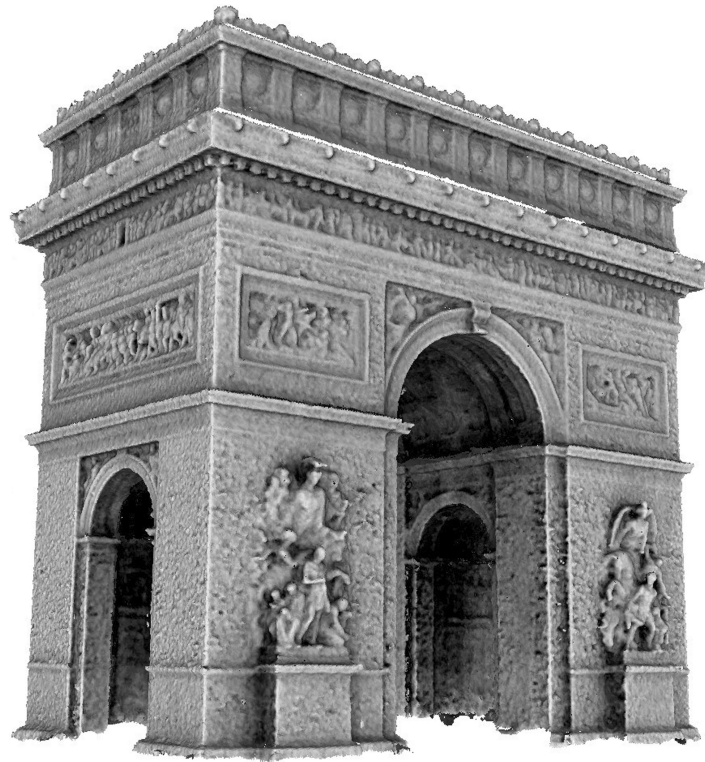
Fig. 7. A 3D model reconstructed from just a sequence of 100 high resolution photos. The reconstruction was performed using the tools developed within the EU IST NoE Epoch .
